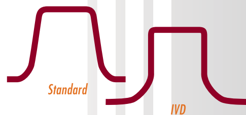
Fig. 11: Comparative rolling diaphragm cross-section
