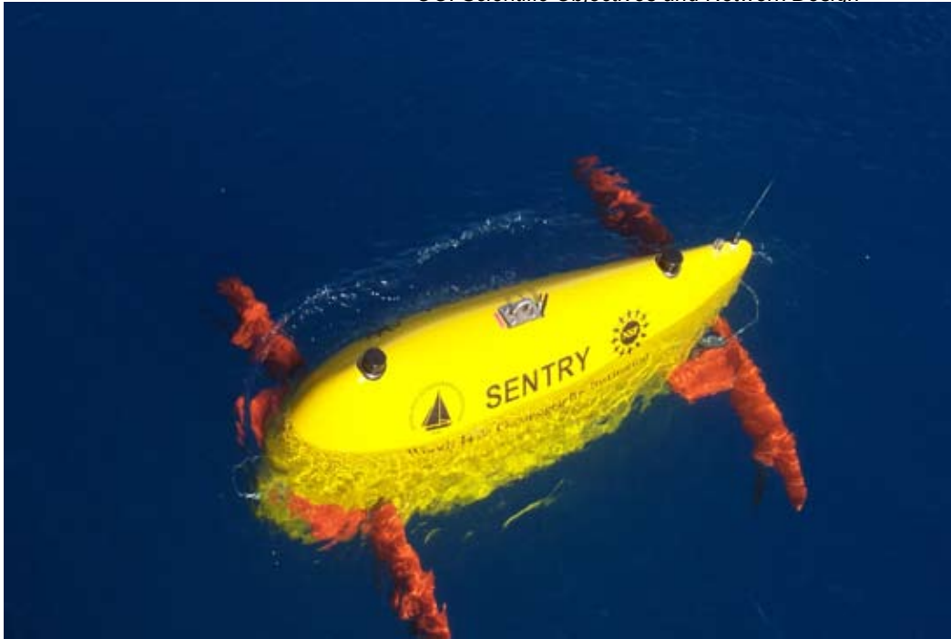
Figure 22. An example of a “next generation” autonomous vehicle that will be a key element of ocean observatory systems for both event response and for characterization of the volume of ocean around an observatory node.
