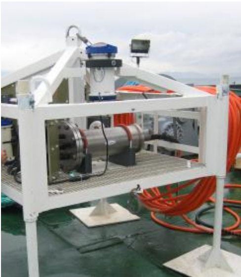
SIIM Mounted on Multi-Instrument Platform
