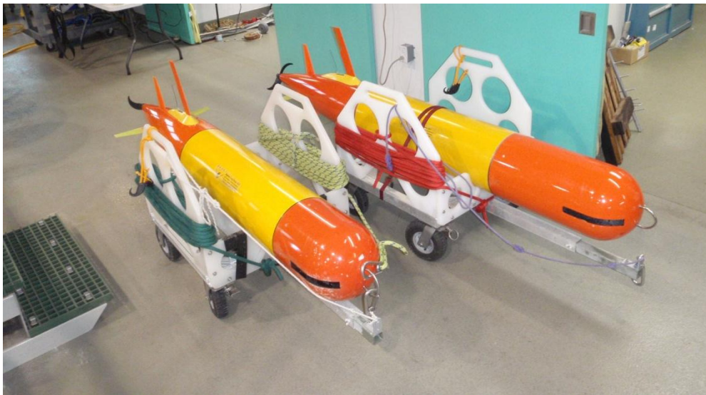
Figure 1 below. The AUVs are about 8 feet long, weigh 220 lbs and use lithium-ion
