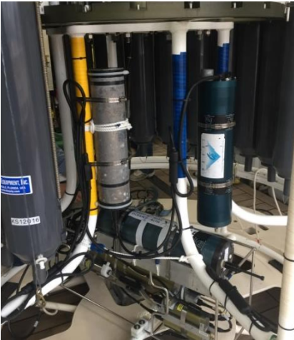
(left) MBARI developed pH (Deep-Sea-Durafet) and nitrate (ISUS) sensors equipped on the CTD rosette for one-meter resolution profiles. (right) Prototype BGC-SUMO that maps high-resolution surface biogeochemistry.
