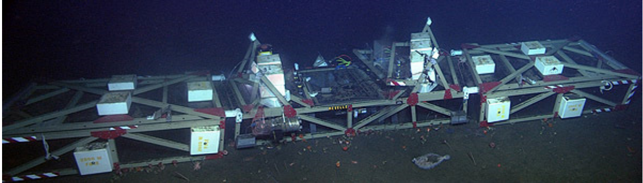
Figure 1. Deep Free Ocean Carbon Enrichment (dpFOCE) system constructed and deployed by MBARI between 2005 and 2011.
