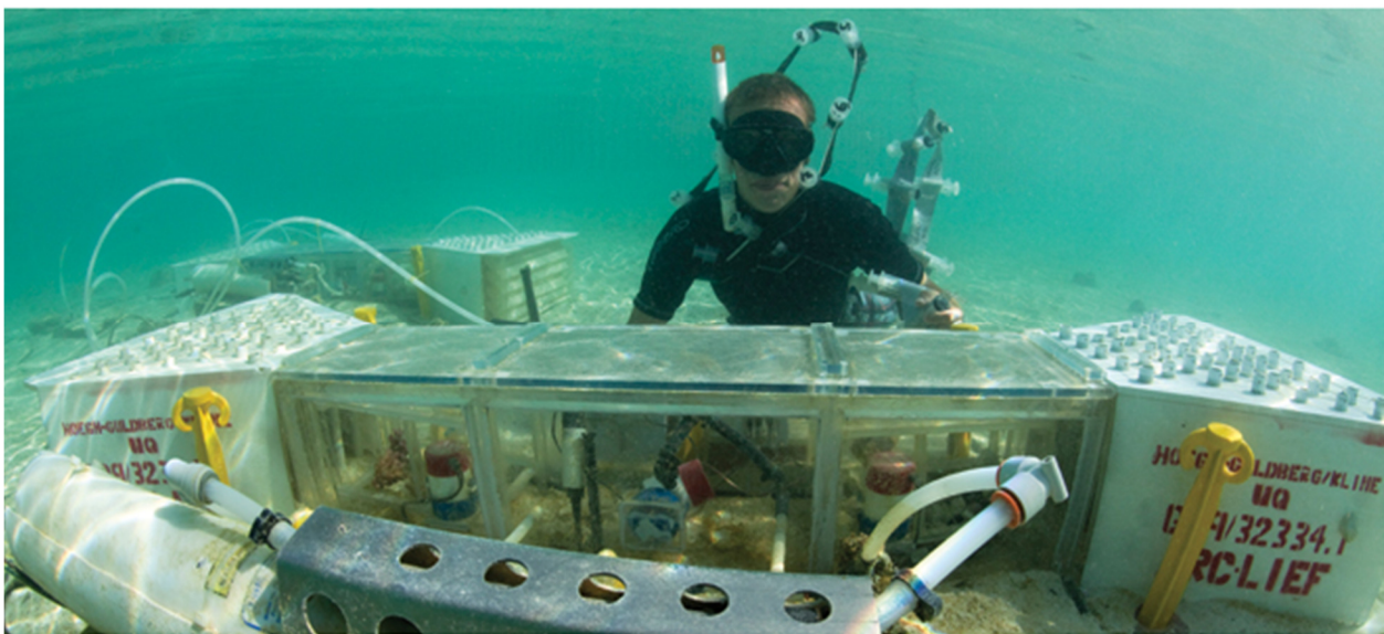
Figure 2. Coral Prototype Free Ocean Carbon Enrichment (cpFOCE) system constructed and deployed in 2009 with the help of MBARI engineers and Dr. Bill Kline.
