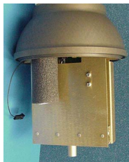
Photo D: Opposite side of Photo C, showing pressure sensor.
