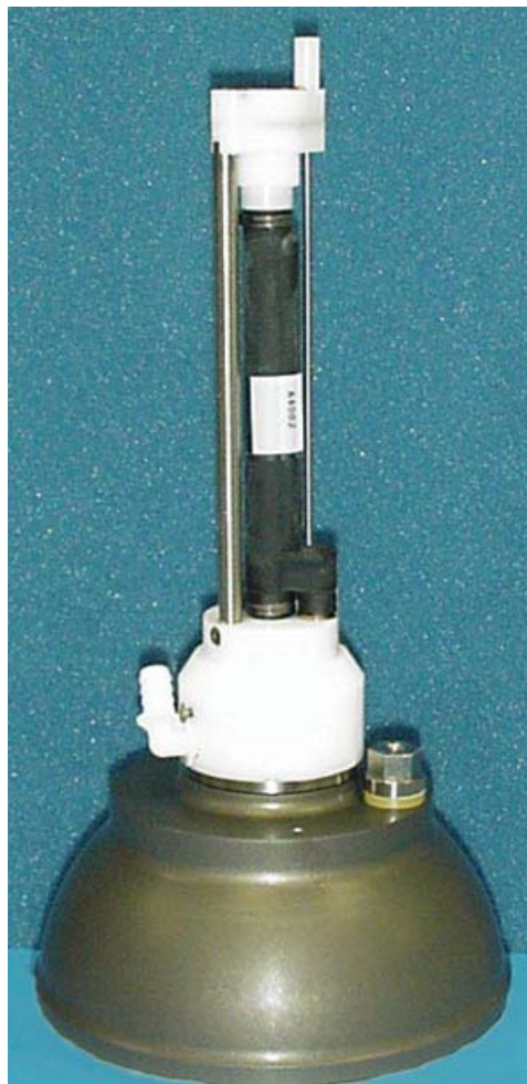
Photo B: Module with guard removed to show conductivity cell.
