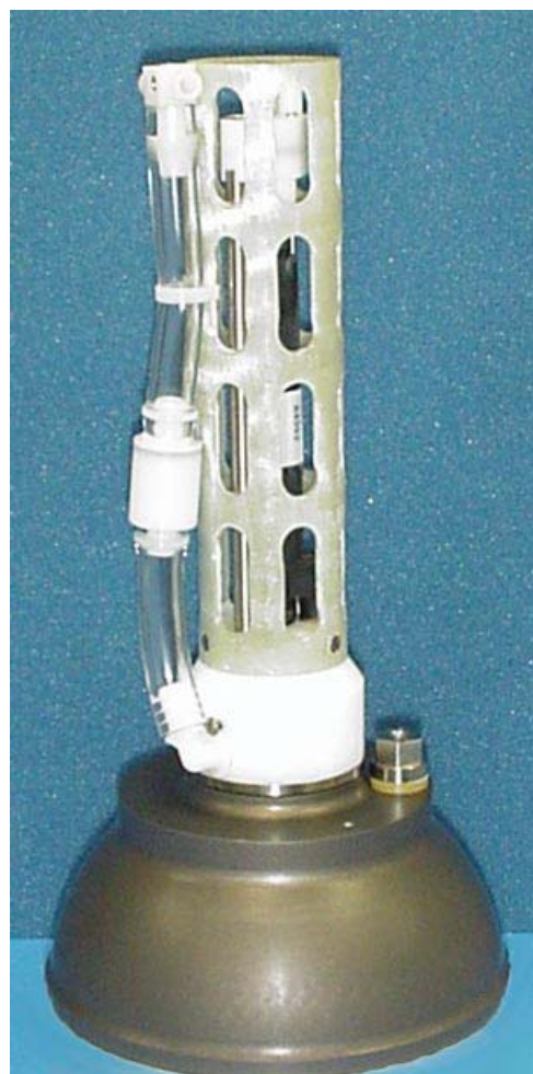
Photo A: Sea-Bird CTD module with guard installed.
