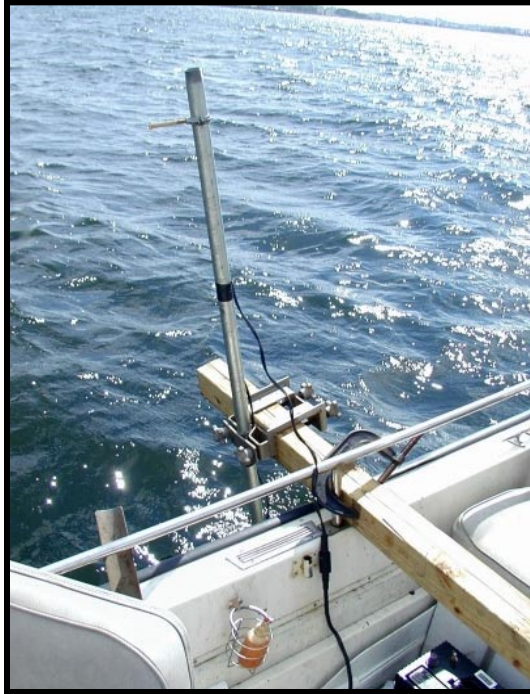
Figure 2-4 Over The Side Transducer Mounting Picture
