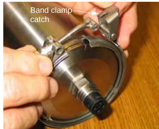
Figure 6-2: Releasing the Band Clamp Catch
