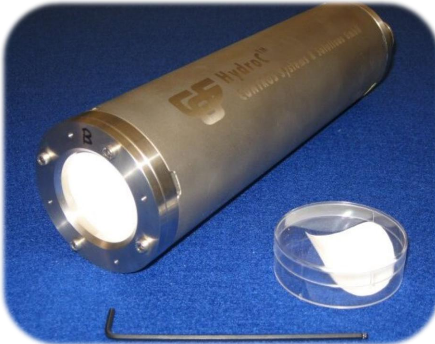
Image 5: The sensor with a new membrane and the 4mm Allen key.
