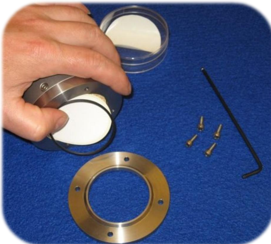
Image 6: Remove the retainer flange and O-ring sealing.
