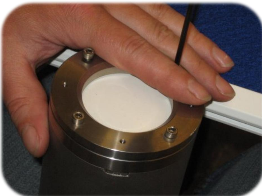
Image 10: Place the retainer flange on its place above the membrane pressed by the O-ring sealing, be sure that everything is on its place; a constant pressure above the retainer flange is needed; be careful to not scratch the membrane surface with any tool/finger. Tighten the screws clockwise and make a final inspection to check if all screws are fixed.
