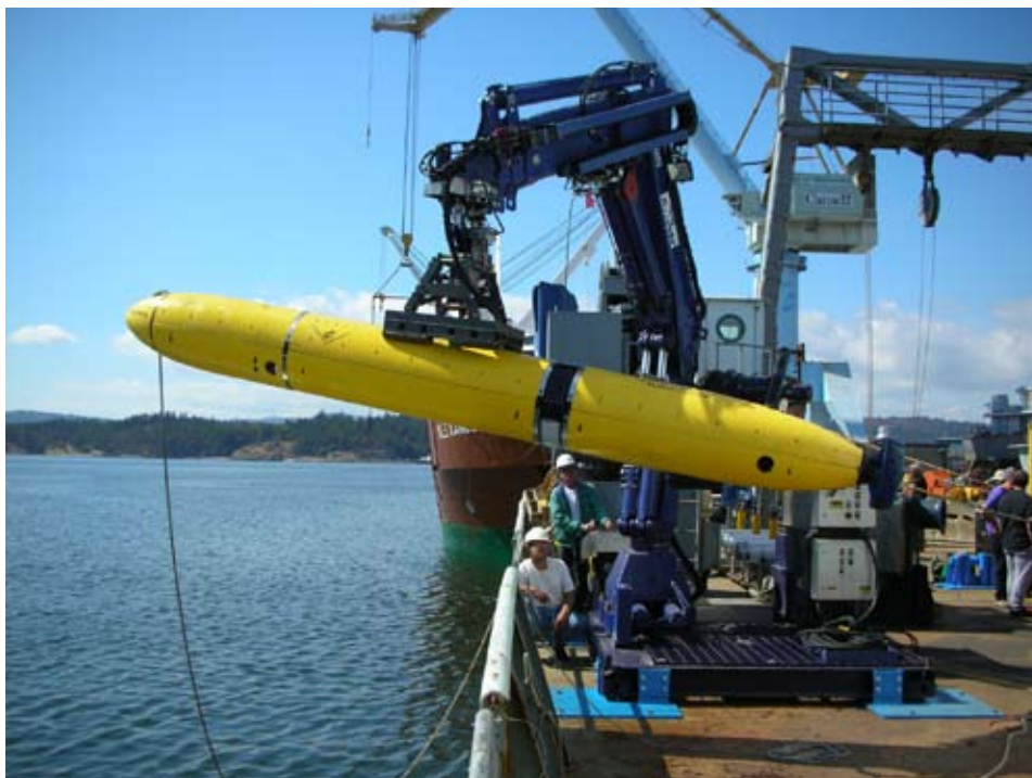
Figure 4. AUV pick using an articulated crane on R/V Thompson.
