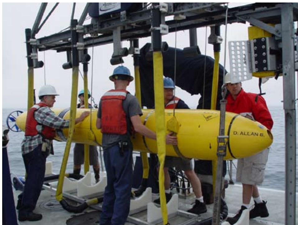
Figure 1. The MBARI AUV D. Allan B. being prepared for deployment from the R/V Zephyr . The Zephyr is equipped with a specialized J-frame crane for AUV launch and recovery over the stern.
