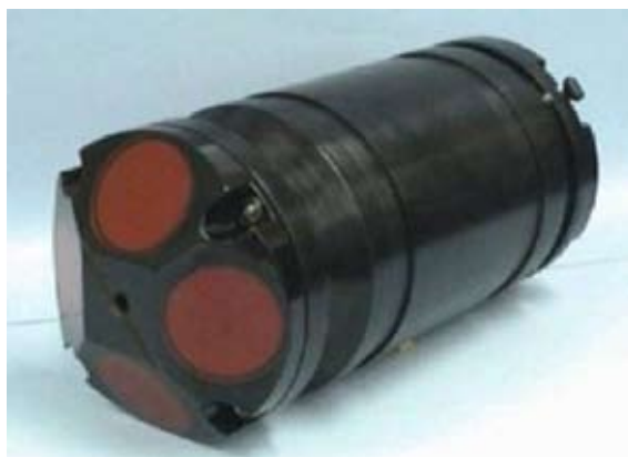
Figure 6. Kearfott Seadevil inertial navigation system (INS) lying on its side. The lower end of the housing consists of a 300 kHz RDI Doppler velocity log (DVL). The aluminum housing encloses both the INS and DVL electronics.
