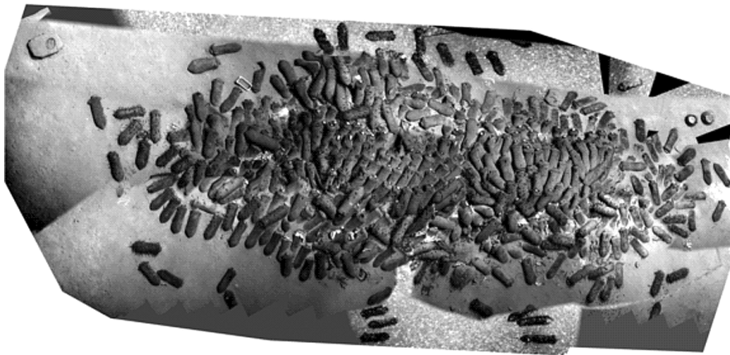
Fig. 19. Final mosaic based on finite element warping of individual strips to a high-altitude low-resolution mosaic of the site. This mosaic highlights the effectiveness of our technique for dealing with terrain effects.
