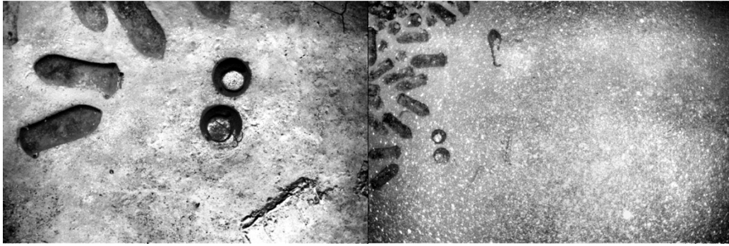
Fig. 3. Effects of backscatter for geometries with small camera-to-light separation. The images of the two cooking pots and amphorae, which are part of a Phoenician shipwreck taken by the Jason ROV from altitudes of 4 m (left image) and 8 m (right image). The area corresponding to the left image is boxed in the right image. Backscatter effects severely limit image quality at the higher altitude.
