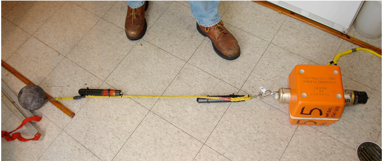
Figure 2. Hydrophone configuration used for initial testing. The two hydrophones (Acousonde B0003A from Greeneridge Sciences) are attached to a 1 m long poly line attached a homer pro beacon and float to a lead ball anchor. The sondes are quite small: 22 cm long and 3.2 cm in diameter. Each can record 16 Hz to 9 kHz acoustic data sampled at 27 kHz for 42 hours.
