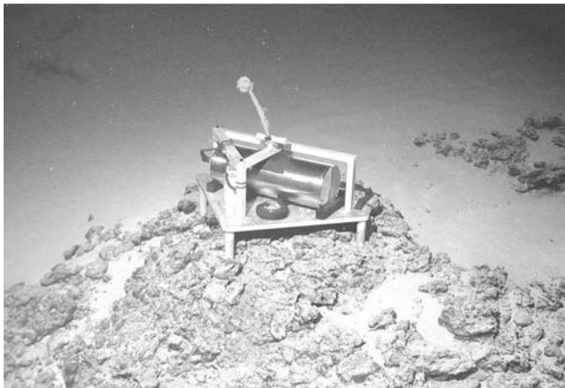
Fig. 8 The OBT in the Logatchev hydrothermal vent field on top of a small rock pile. For installation with the ROV a floating rope was tied on the OBT above the center of mass. On the left side of the OBT frame an additional aluminium L-profil holds a miniaturized temperature logger. Steep slopes (here in the foreground of the photo) and a sediment cover of about 1 m thickness (here in the background) characterize the area. Ripples on the sea-floor in the background indicate currents
