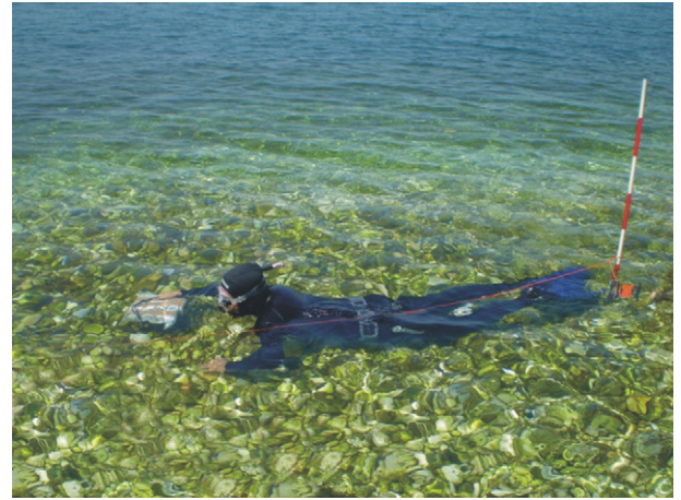
Fig. 7. A snapshot of the recovery campaign: when a pebble is detected, the identification code of the tag pops up on the screen of the laptop placed on a small boat. An acoustic signal aids in the retrieval operation. The diver uses a rope tied to poles to follow predetermined paths. In this way, he avoids patrolling the same area multiple times.
