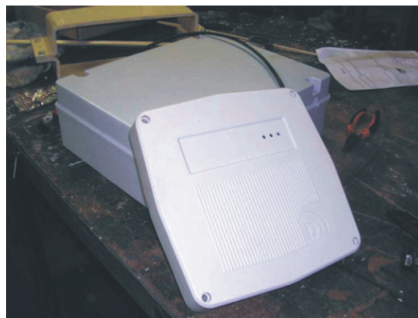
Fig. 1. The CORE-125 reader chosen as the operating antenna. It is connected to a pair of 12 V–7 A batteries and the laptop computer. These long-life batteries allow several hours of fieldwork without further charge.
