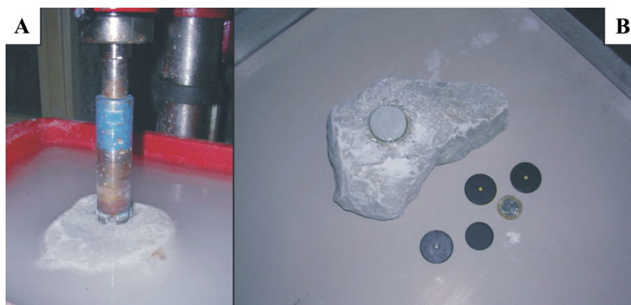
Fig. 2. A core drill (A) was used to drill precise and sharp holes in the pebbles. After preparation (B), the pebble's shape and weight are not significantly modified. The black disks represent the transponders used during the experiment.
