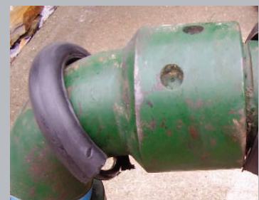
Variation of RFID "Frac-Tag" on valve (left) and swivel (right)
