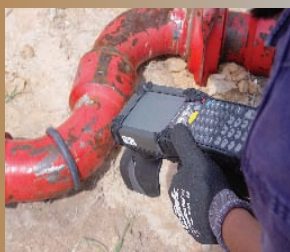
RFID Scanner Reading "Frac-Tag"
