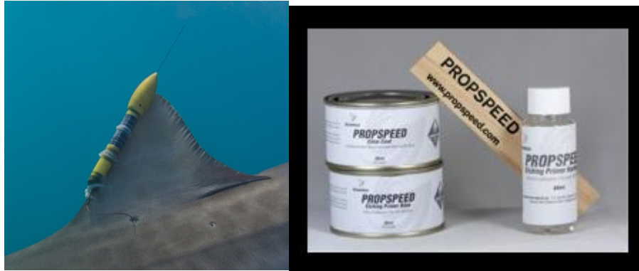
Figure 8.1 (left) shows a Propspeed coated tag in action and (right) Propspeed antifoulant paint kit.
