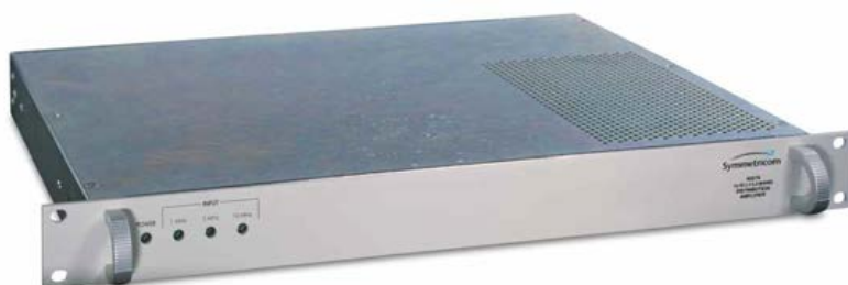
4037A 1x16 L1/L2-Band Distribution Amplifier
