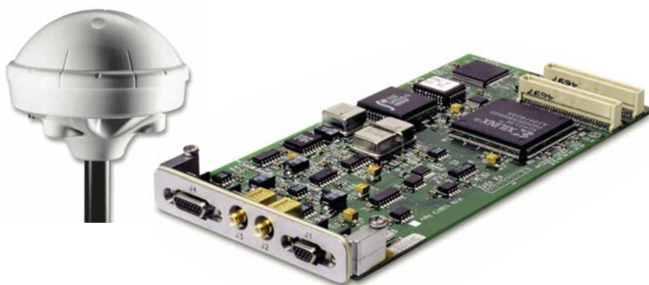
PMC Time & Frequency Processor (shown with optional antenna/receiver, bc637PMC)
