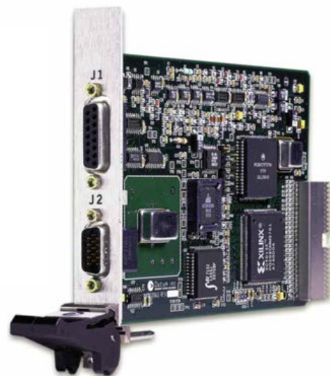
CPCI Time & Frequency Processor (shown with optional antenna/receiver, bc637CPCI)
