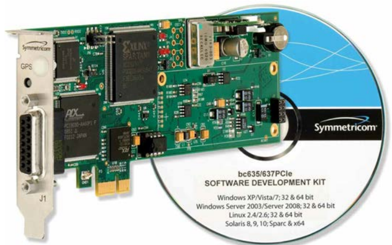
bc635PCle Time & Frequency Processor & Included SDKs/Drivers
