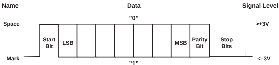
Figure 6–82. The RS232 Format (Levels on the Transmission Line)
