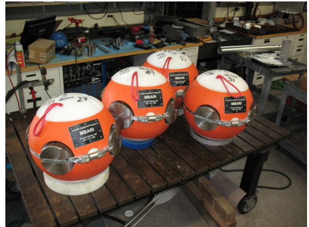
Figure 1 –BEDs with new dropweight system just prior to deployment.
