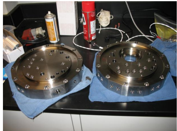
Fig. 4 Sample and Exhaust bulkhead plates for DWSM, made from 6Al4V titanium, Exhaust plate on right. Over 100 hours of CNC machining was required, and helical mill threading was used for the 80 threaded holes.
