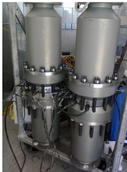
Fig. 5 DWSM assembly with flanges and jacket bolts for 20 MPa pressure validation prior to deployment. The jacket bolts are pre-tensioned to maintain seal integrity when internally pressurized.
