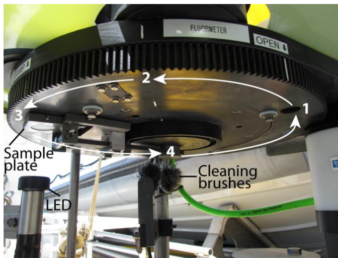
Figure 3. Carousel assembly viewed from below. Sample bottles have been replaced with a white, translucent sample collection plate, which is rotated through collection (1), fluorometry (2), and imaging (3) stations. A light-emitting diode (LED) light at the lower-left illuminates the sample from below for imaging. After the sample has been analyzed, it is discarded and the sample plate is passed through a set of cleaning brushes (4). The clean sample plate is then rotated back to the base of the funnel to begin collecting the next sample.
