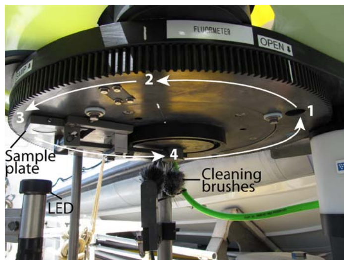
Fig. 3. Carousel assembly viewed from below. Sample bottles have been replaced with a white, translucent sample collection plate, which is rotated through collection (1), fluorometry (2), and imaging (3) stations. A light-emitting diode (LED) light at the lower-left illuminates the sample from below for imaging. After the sample has been analyzed, it is discarded and the sample plate is passed through a set of cleaning brushes (4). The clean sample plate is then rotated back to the base of the funnel to begin collecting the next sample. Alternatively, the carousel can be left in a flow-through position such that the sample plate is not beneath the base of the funnel, and the sinking particulate matter flows through a hole in the carousel plate without being collected. This allows the sample analysis interval to be longer than the collection time to avoid accumulating too much material on the sample plate during long analysis intervals or during times of heavy particulate flux. For example, a sample can be collected for 2 h, followed by a 4-h flow-through mode before collecting another 2-h sample.
