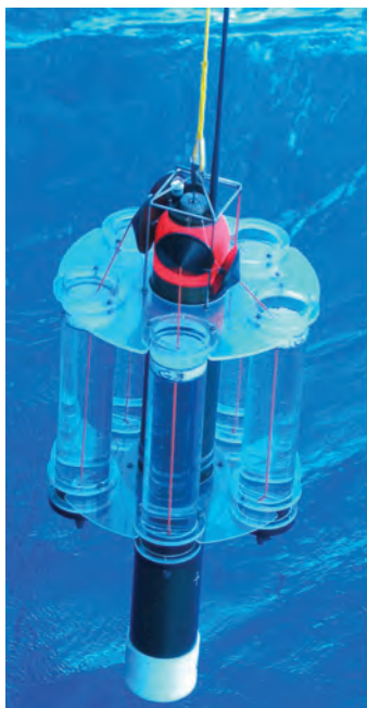
Figure 2.3. Photos of two neutrally buoyant traps used successfully to collect sinking particles in the ocean. (a) NBST (Valdes and Price, 2000; Valdes and Buesseler, 2006). (b) PELAGRA (Lampitt et al. , 2004).
