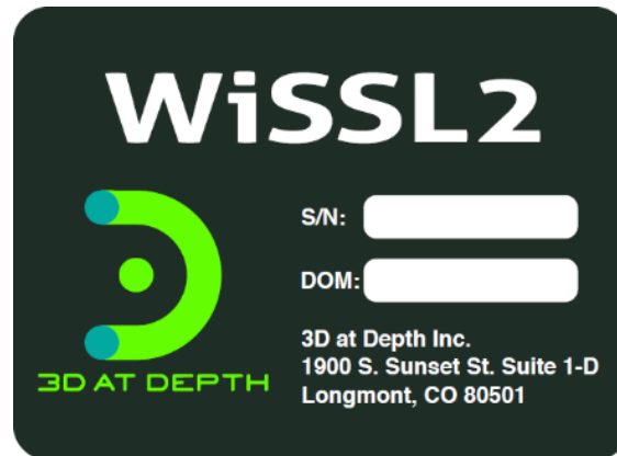
Figure 5 - Identification labels for the WiSSL-Gen2 family of sensors. Each serial number (S/N) is tracked at the factory for the month, year, and location of manufacture.
