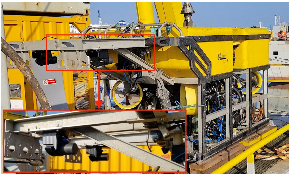
Figure 19. Dual WBMS Basic on a STD Quasar ROV with IXBLUE ROVINS
