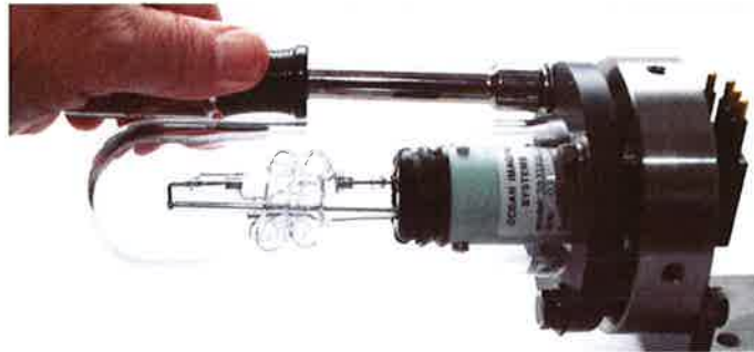
Figure 5.4 Flash Head Retaining Bolt Removal
