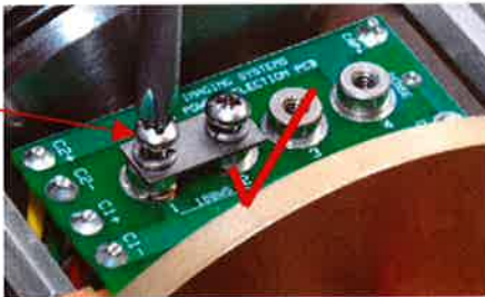
Figure 3.6 When removing shunts, loosen both screws before removing either completely. When installing shunts, install both screws partially before tightening.
