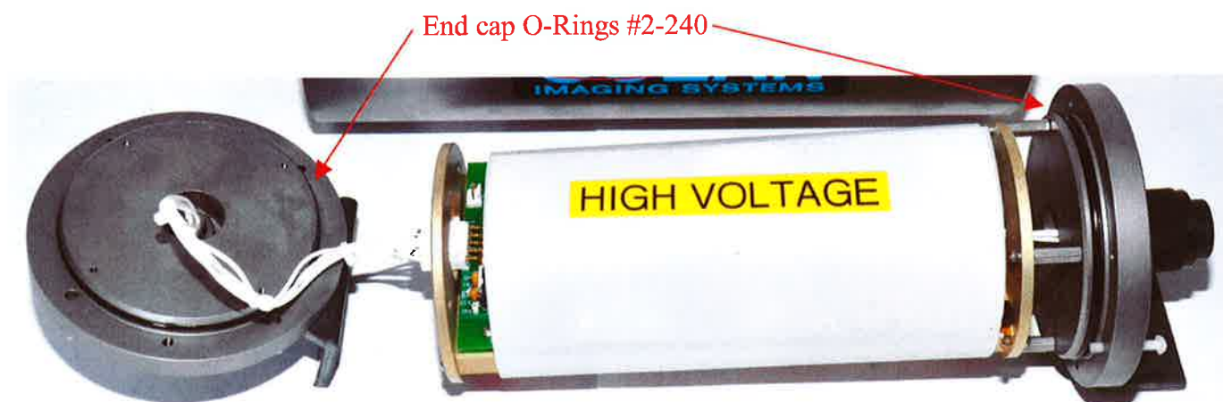
Figure 5.3 Chassis Assembly Shown With Housing Removed
