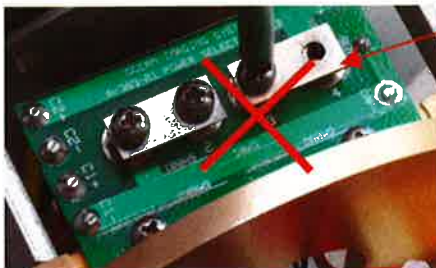
Figure 3.7 DO NOT remove one screw completely, before loosening both.
