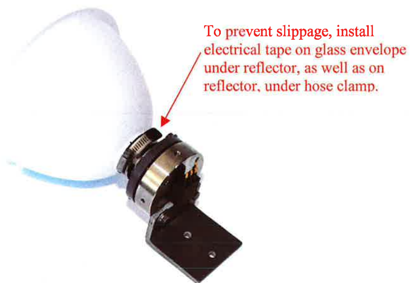
Figure 5.6 Remote Flash Head with Reflector Installed
