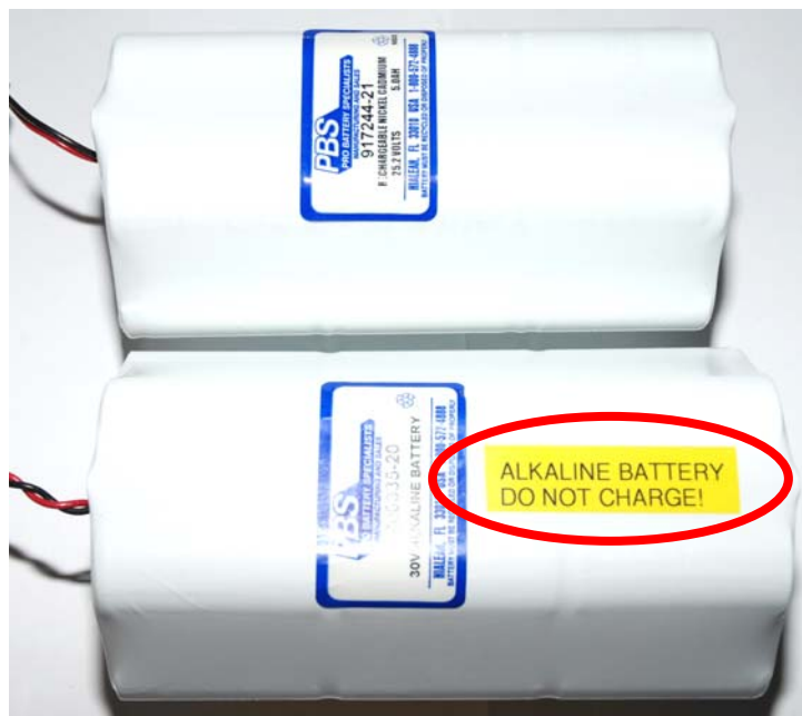
Figure 6.0 Ni-Cad Battery Above, and Alkaline Battery Below
