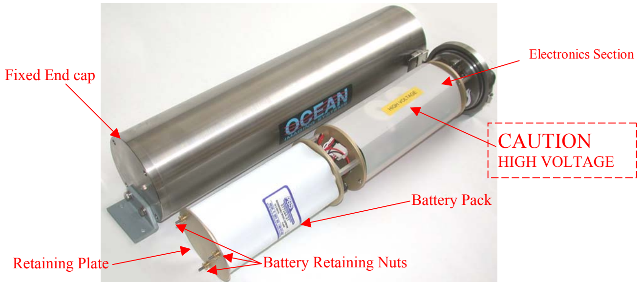
Figure 5.2 Chassis Shown Removed From Housing
