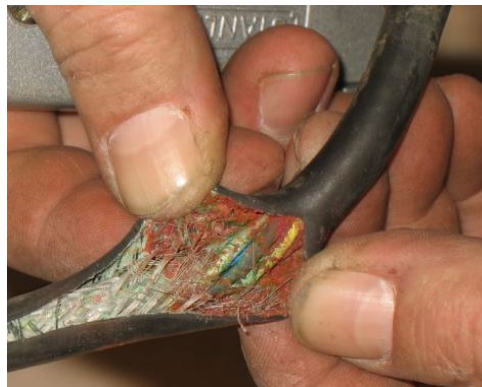
Figure 20. Do not use Zip-Ties Directly on Cables
