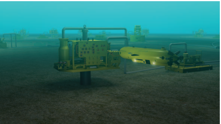
High bandwidth through-water communications using Free Space Optical technology will enable video transmission and tetherless control of AUVs for inspection and light intervention operations.
