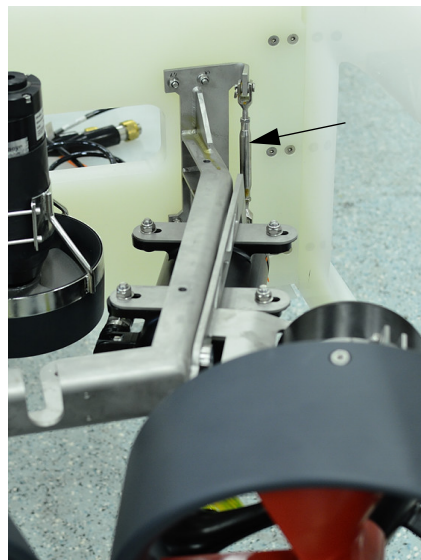
Figure. 6.25 Thruster Tilt Adjustment. The arrow points at a turnbuckle.
