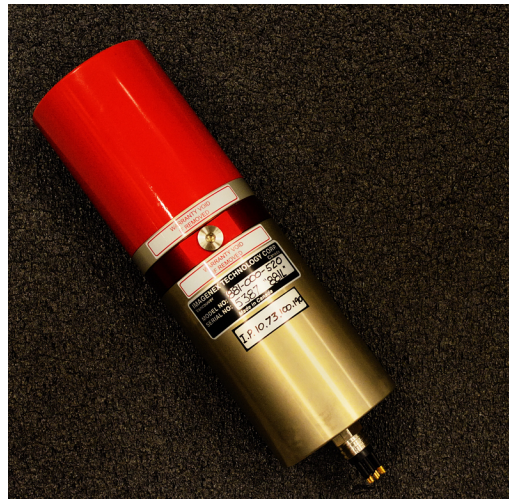
Figure. 1.12 Sonar Imagenex 881L
