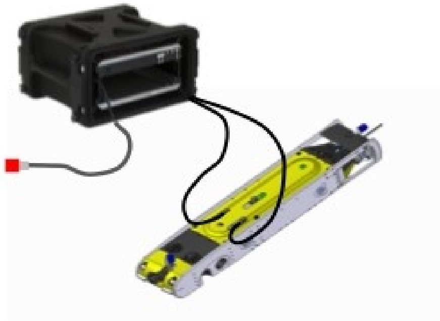
Figure. 7.8 Battery charger connection
