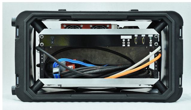
Figure. 1.16 Battery Charger mounted in dedicated box
