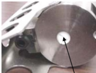
Standard pressure sensor port plug. (Note: Photo is SBE 37-SM. Pressure port details are similar for all instruments included in this application note)
