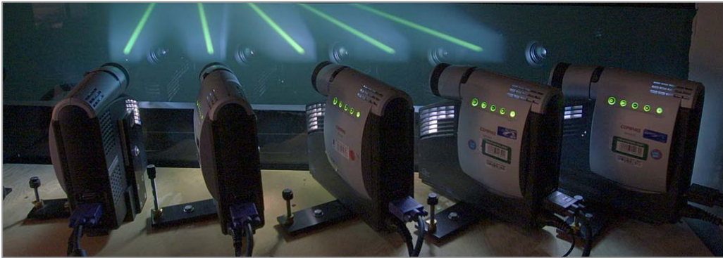
Figure 4. Experimental setup using multiple illumination sources.
