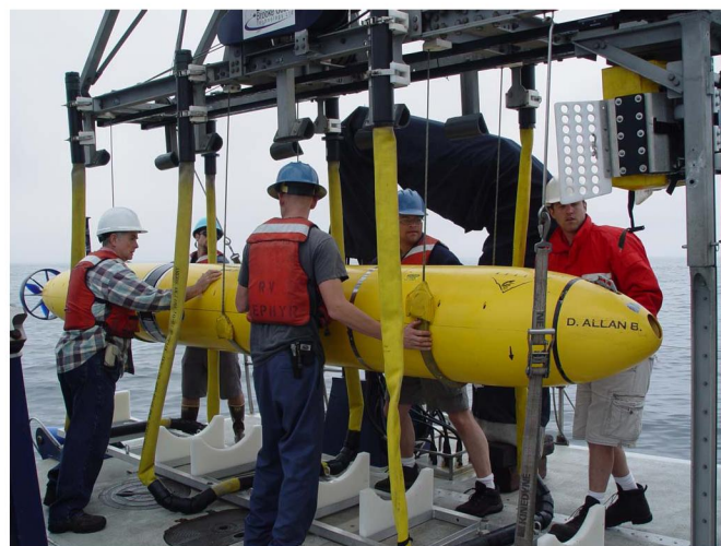
Fig. 1. The MBARI Mapping AUV being prepared for deployment from the R/V Zephyr . This 21" diameter, 17.2' long vehicle includes a 200 kHz multibeam, 110 kHz and 410 kHz chirp sidescans, and 2-16 kHz subbottom profiler.
