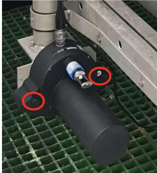
Figure 13. WBMS mounted without bracket
