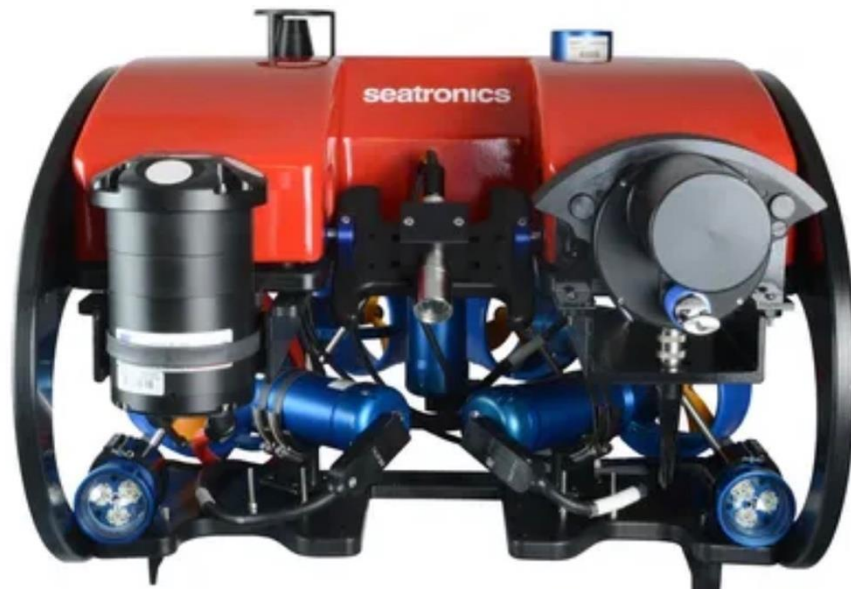
Figure 16. Up looking WBMS Bathy on Seatronics
