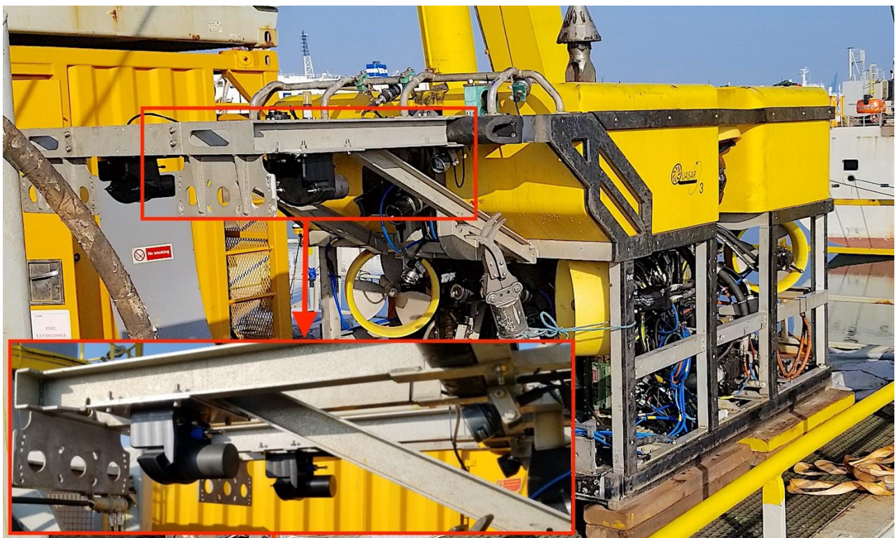
Figure 15. Dual WBMS Basic on a STD Quasar ROV with IXBLUE ROVINS
