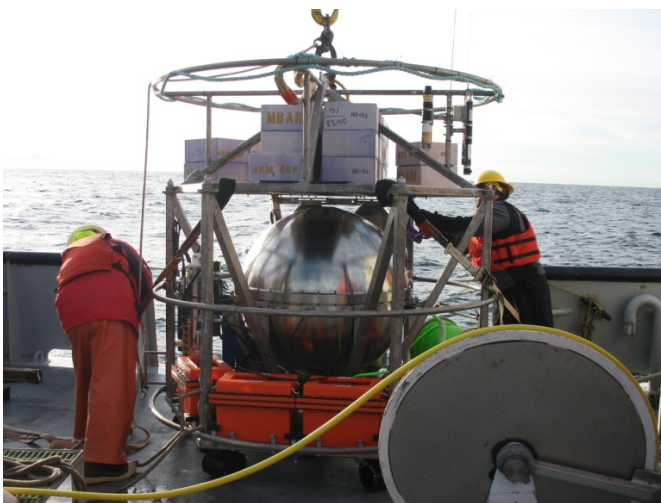
Fig. 11. The sphere, mounted in a freefall benthic lander, is being readied for deployment in the Monterey Canyon from the R/V Point Lobos.
