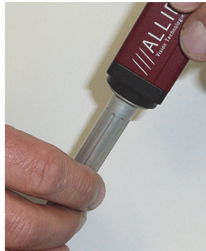
Figure 3: Removing IR cut filter/protection glass using special tool (E9020001)
