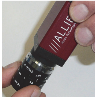
Figure 1: Illustration of camera orientation when removing lens or dust cap
