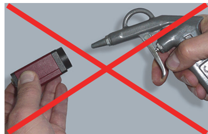
Figure 6: Don't use compressed air
