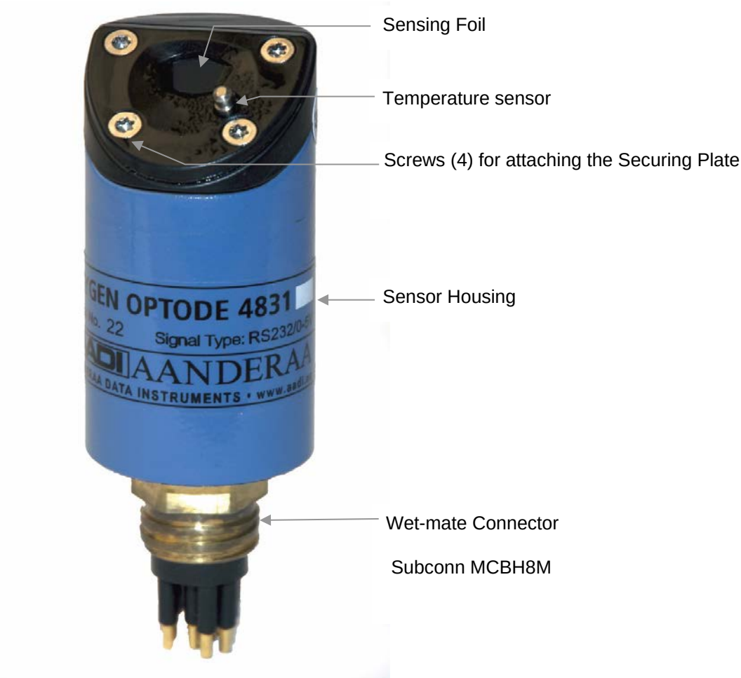
Figure 1-2 Illustration of the Oxygen Optode 4831
