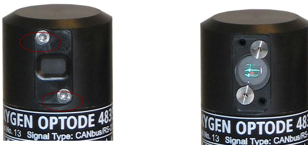
Figure 6-4 Removing the securing plate and change the sensing foil.
