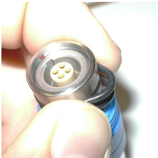
Close-up of how to properly remove exterior O-rings from a device
