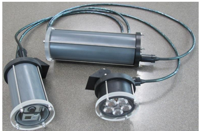
Fig. 1. SeeStar is composed of a camera module (left), a battery module (top) and a LED lighting module (bottom). It can easily be adapted and mounted on various platforms.
