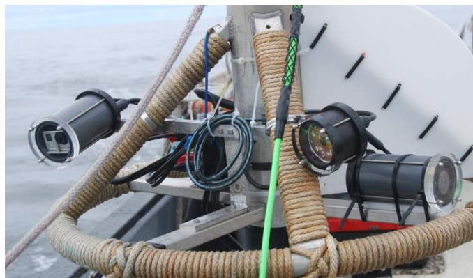
Fig. 8. SeeStar was mounted on a lander and lowered to the sea floor in multiple locations. The camera module (left), the LED module (center right) and the battery module (right) can easily be mounted on various platforms.
