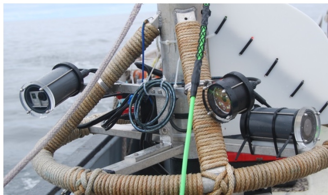
Fig. 8. SeeStar was mounted on a lander and lowered to the sea floor in multiple locations. The camera module (left), the LED module (center right) and the battery module (right) can easily be mounted on various platforms.
