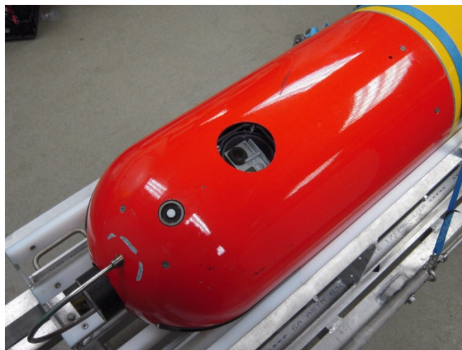
Fig. 10. SeeStar was mounted inside the nose of a long range autonomous underwater vehicle, with the camera facing upwards. The images are used to count jellyfish in the water column.
