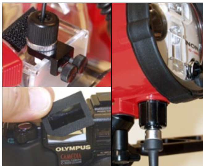
INON Details Left Top: Cable attachment to housing diffuser. Left Bottom: Film mask blocks visible light, but passes IR. Right: Secure connection to strobe.
