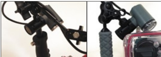
Ikelite tray and arm system has a fixed post for the controllers (left). With the triple clamp, the aim of the controller is moved with every arm adjustment.
