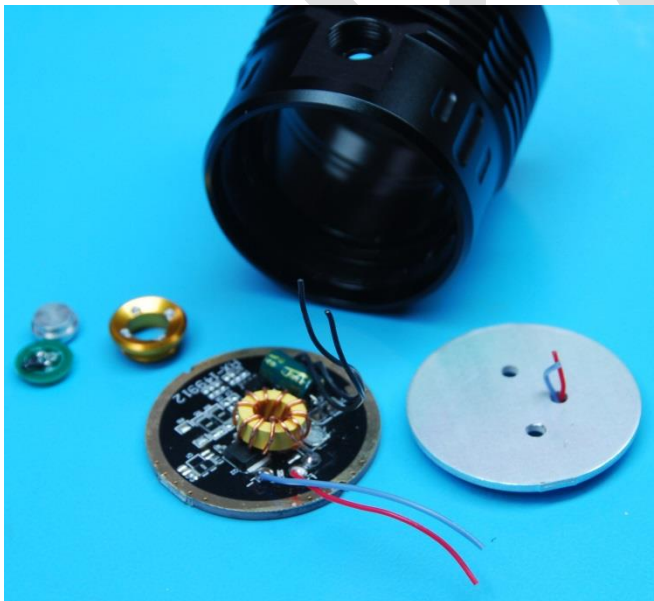
Figure 10: The driver board (left) and the LED board (right) removed from the flashlight
