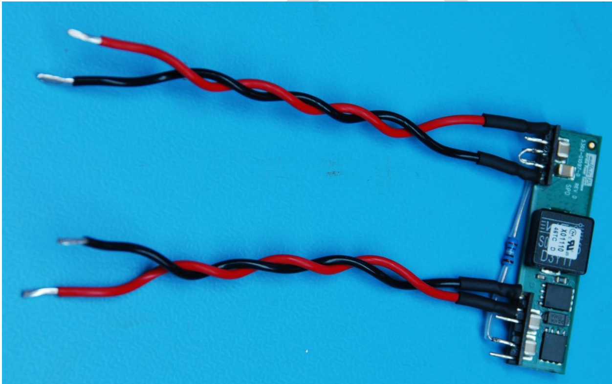
Figure 12: The DC-DC converter wired
