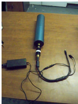
SBP-2 battery pack connected to ACDC-U charger via FCBL-A adapter cable and 6-pin/8-pin converter
