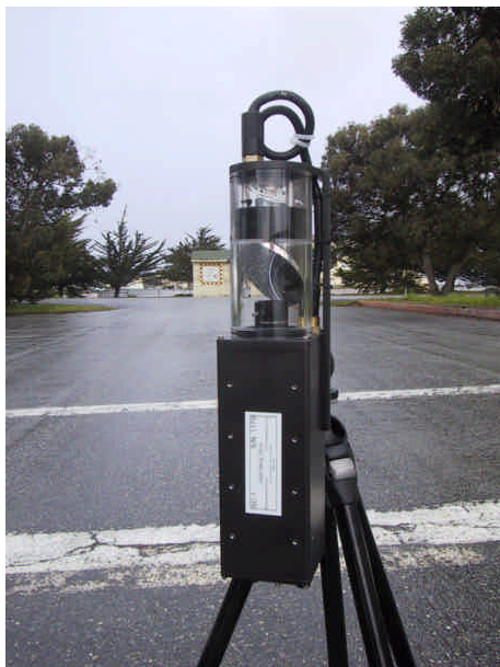
Custom Housings: With 360° rotating mirror (left), with dome port (right)
