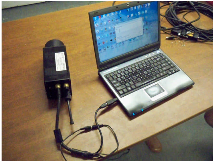
Image retrieval via Firewire: Connect the camera to a Firewire port on your PC via the short adapter cable. The adapter cable includes a Firewire regular to mini connector adapter. Use as suitable for your PC. If the PC doesn't have a Firewire port, adapter cards are available. Use the Image_Retrieval software.
