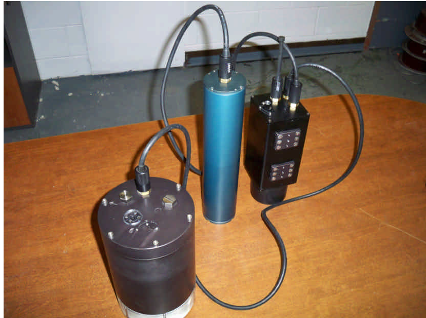
Camera autonomous station without surface link: The camera is now powered by the SBP-2 battery pack (blue cylinder) and the surface umbilical is not used.
