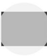
Partial Frame: Image circle < diagonal of the sensor
