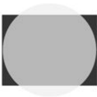
Horizontal Frame: Image circle <= width and > height of the sensor
