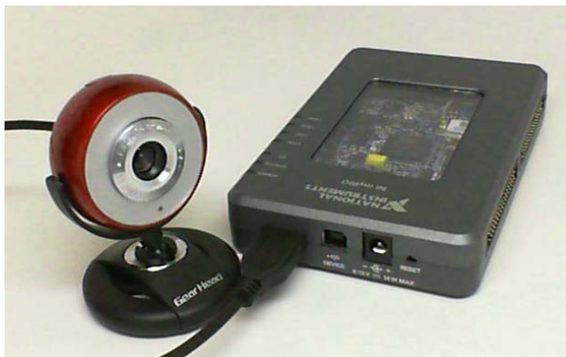
Figure 36.1: webcam connected to NI myRIO USB port.
