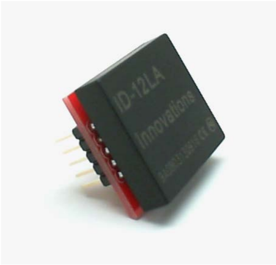
Figure 38.2: RFID reader, breakout board, and headers after soldering.
