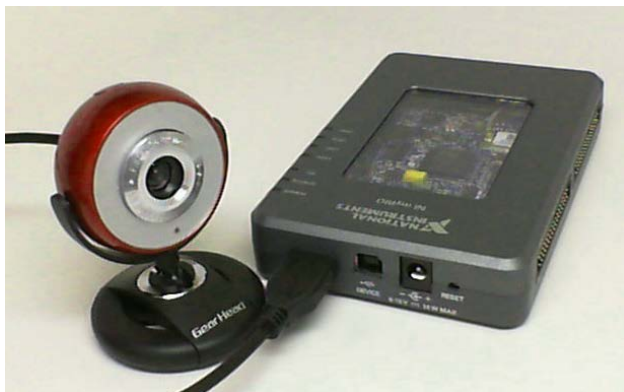
Figure 36.1: webcam connected to NI myRIO USB port.
