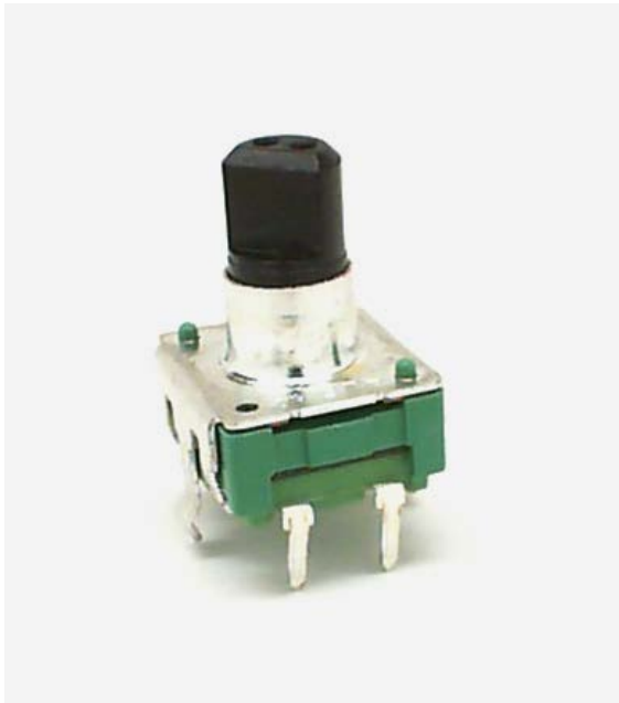
Figure 4.1: NI myRIO Starter Kit pushbutton switch integrated with rotary encoder.
