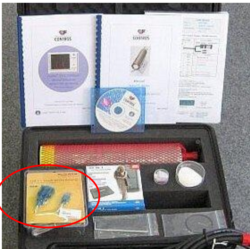
Image 1: A RS232-USB Adapter is supplied from CONTROS. Use the CD to install the driver.
