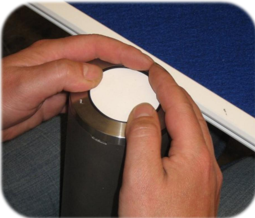
Image 9: The now stretched O-ring sealing can be pushed on the membrane to fix it. Do not press on the membrane surface; do not rub over the surface of the membrane. Be sure that the membrane has no folds on it.
