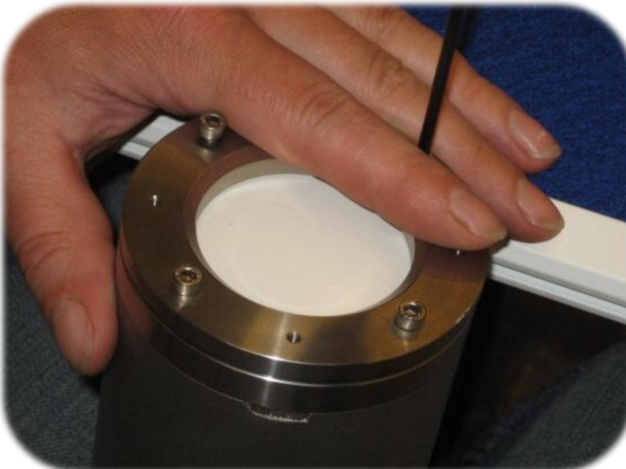
Image 10: Place the clamping ring on its place above the membrane pressed by the O-ring sealing. Be sure that everything is properly placed; a constant pressure to the clamping ring is needed; be careful to not scratch the membrane surface with any tool/finger. Tighten the screws clockwise and make a final inspection to check if all screws are fixed.
