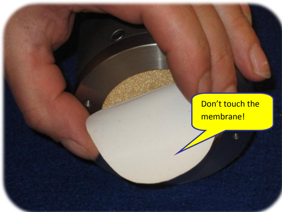
Image 7: Place the new membrane on the sinter metal.
