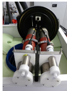
Image 4: Sensor with flow head and SeaBird pump
