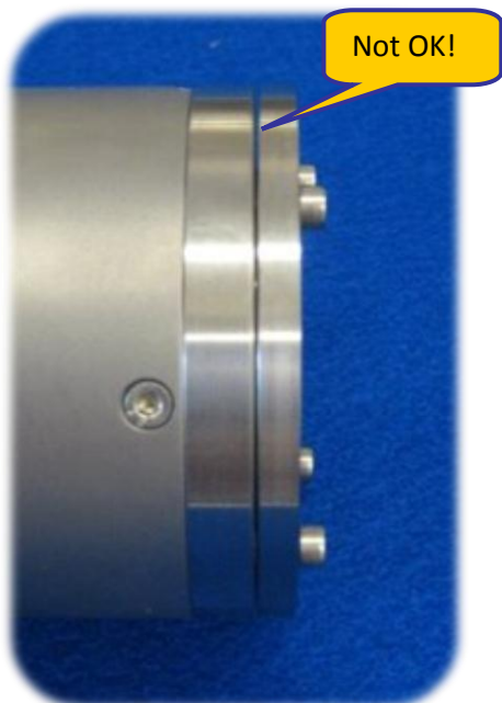
Image 11: A small gap shows the non-constant pressure on the O-ring sealing. Check the O-ring to be well fitted and try again. Tighten the screws clockwise until they are completely fixed.
