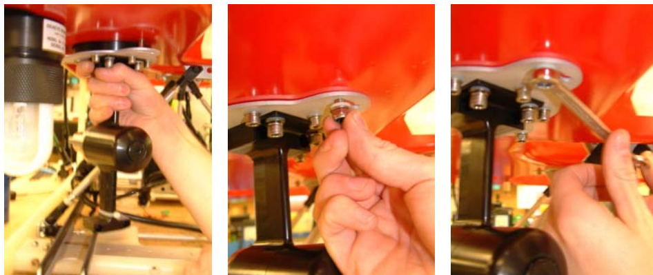
Fig. 25. Fitting the Forward Thruster
