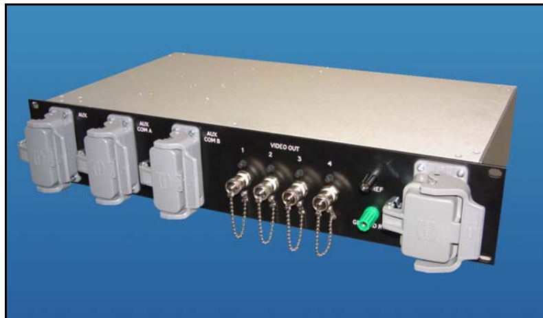
Fig. 6. Surface Control Unit
