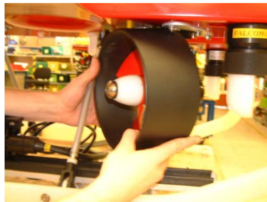
Fig. 19. Thruster Nozzle Removal
