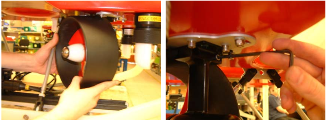
Fig. 29. Thruster Nozzle Fitment
