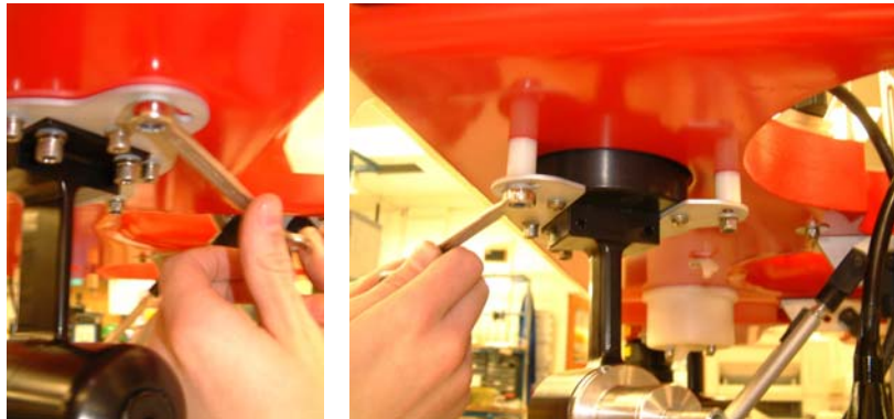
Fig. 21. Thruster Mounting Plate Removal
