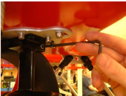
Fig. 19. Thruster Nozzle Removal
