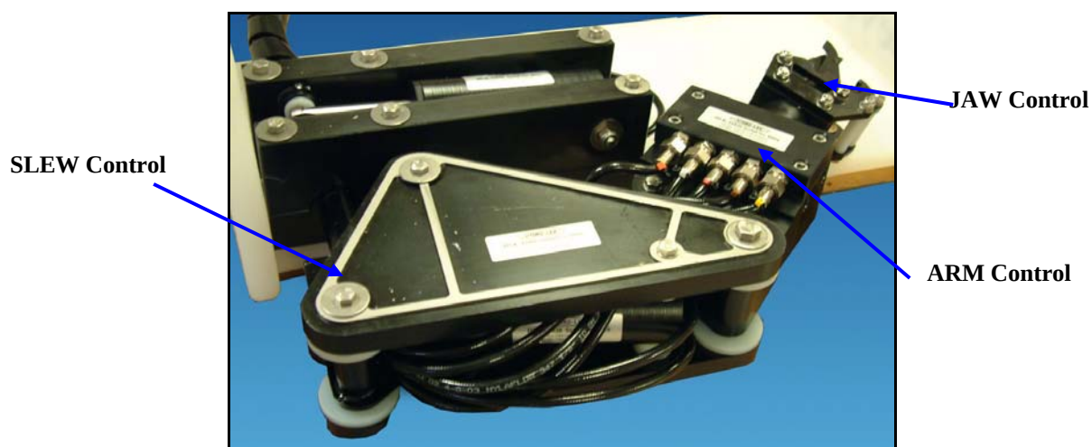
Fig. 4. Manipulator Controlled Parts
