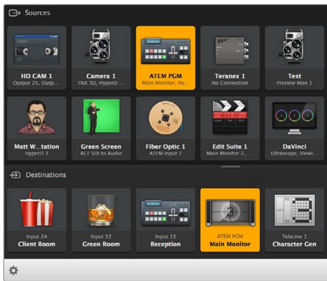
Blackmagic Videohub Software Control lets you manage and route multiple sources and destinations using one single control panel
